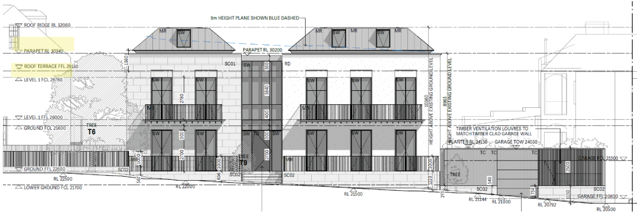
Figure 6: Proposed front elevation at 38 Lower Fort Street showing the 9m height plane in dashed blue and the existing height above ground-level in the north-eastern corner of the proposed building. (Source: Andrew Burns Architecture / Tasman Storey Architect)
